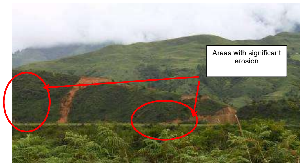
Fig: 8.41 Road construction activities above Mechuka Bridge leading to soil erosion
